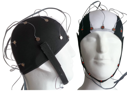
Fig. 3. HapticHead for vibrotactile feedback around the head [26].
