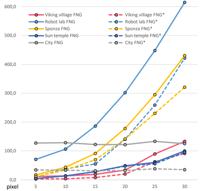
Fig. 16. Average false negative pixel count per frame for all possible views. FNG (solid lines) show results with unreliable triangles; FNG* (dashed lines) shows results without unreliable triangles. When applying the cut-off suggested by Wonka et al. [2006] of roughly 100 pixels, a viewcell size of 15-20 cm can usually be supported without any noticeable errors.
