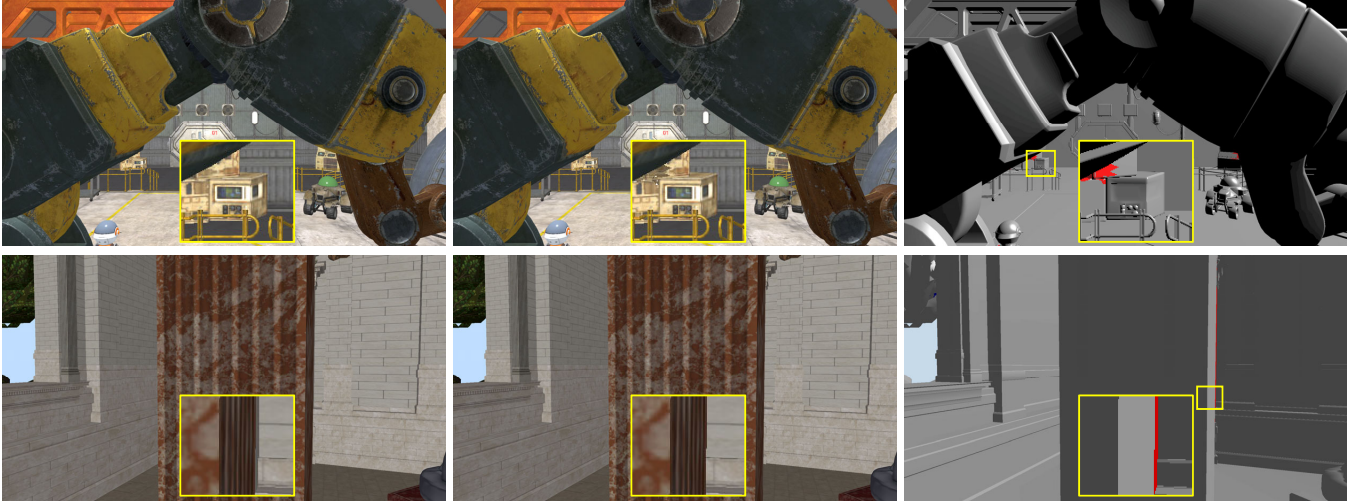
Fig. 17. Challenging situations in Robot lab (top row, 210 false negative pixels) and Sun temple (bottom row, 344 false negative pixels). In each row, the left column shows the full scene; the middle column shows the PVS computed by TR, and the right hand side highlights false negative pixels in red. The differences to the full scene are not immediately apparent in the PVS rendering.
