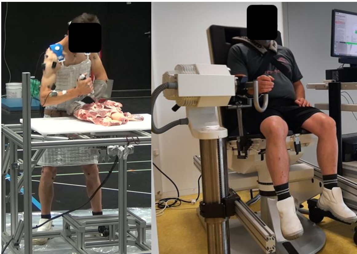
127 Figure 1: (a) Marker placement on the subject (markers on the right side are shown in orange, while 128 those on the left side and centre are shown in blue). Additionally, markers located on the knife and 129 table (one marker on the table was on the opposite and is not visible in the photo). The coordinate 130 system on the knife shows the force sensor origin. (b) a subject in action during a pork belly cutting 131 trial (left), and a maximal isometric wrist radial deviation strength test (right).
