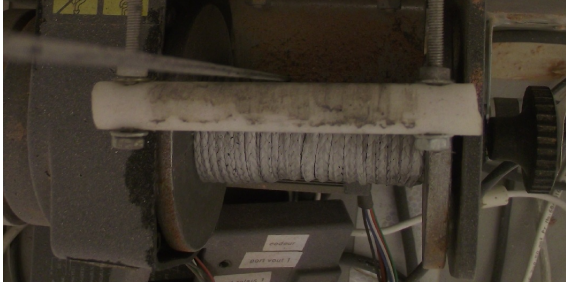
Fig. 9. The cable 4 coiling over a two months period.
