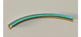
Fig. 11. Image-based measurement of the curvature  $\kappa$ .
