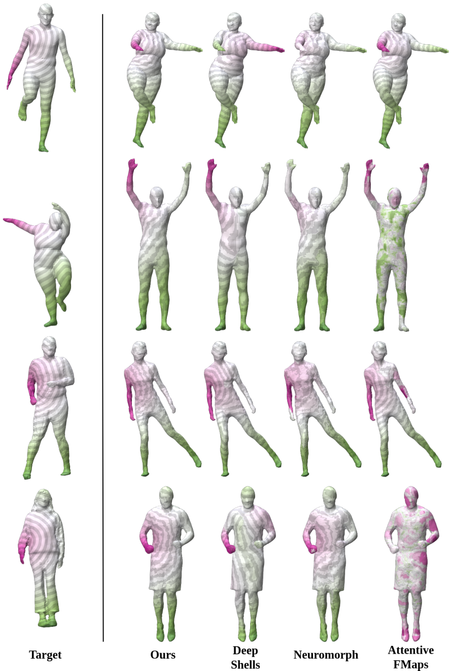
Figure 9: Comparisons with Deep Shells [12], Neuromorph [13] and AttentiveFMaps [14] on pre-processed human meshes (first and second rows) and on raw human 3D scans (third and fourth rows). Each point on the target mesh (left) is assigned a color, which is transferred to the source mesh (right) using the correspondences estimated by the different methods.
