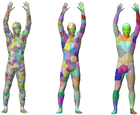
Figure 3: Example of surface patches. From left to right : 800, 200 and 50 patches along with their centers on a mesh with \approx 13k vertices.
