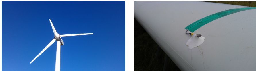
Fig. 1. Vestas V27 wind turbine (left). V27 blade with an accelerometer attached (right).
