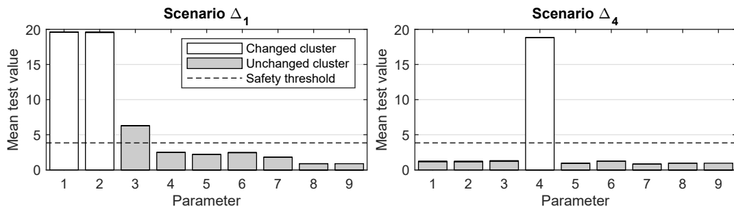
Figure 3: Mean of the minmax localization test statistic for two selected damage scenarios and numerical data
