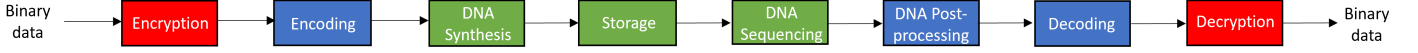
Fig. 1. A common DNA storage chain with its digital (blue) and biological (green) functionalities. Encryption (red) is used to ensure data confidentiality.
