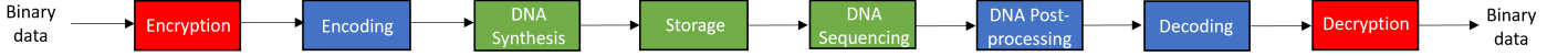
Fig. 1. A common DNA storage chain with its digital (blue) and biological (green) functionalities. Encryption (red) is used to ensure data confidentiality.
