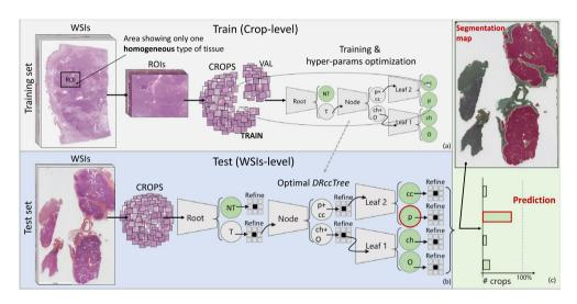
Figure 2. Overview of the proposed ExpertDT. The training phase is based on homogeneous regions depicting the same type of tissue, a-priori identified by a pathologist (a). On the contrary, the testing phase involves the whole WSI (b). Note that the final classification at patient-level comes from a majority voting among the predicted tiles associated to the same subject (c).
