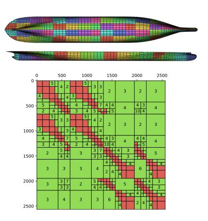
Figure 11: Above: Top and side view of the ship hull mesh where panels colors correspond to the 60 clusters of panels composing the mesh. Below: Resulting  $\mathcal{H}$ -matrix for the S matrix with a density of  $\sim$  21% where red blocks are fully stored in memory and green blocks are low-rank blocks with a rank corresponding to the number displayed in the block.
