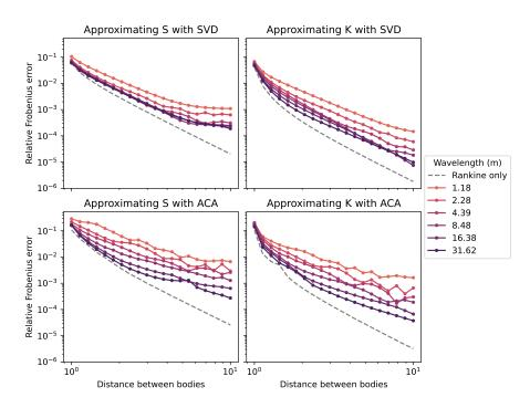
Figure 4: Relative Frobenius error between the full matrix and the low-rank compressed matrix as a function of the distance between the two bodies, for two methods of low-rank compression (SVD and ACA) and two BEM matrices (S and K), for several wavelengths (colored lines) as well as for the Rankine  $1/||x-\xi||$  kernel (dashed gray line).
