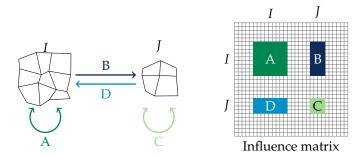
Figure 1: Schematic representation of the matrix blocks encoding the interaction between two sets of panels. Blocks B and D might be approximated by low-rank matrices.
