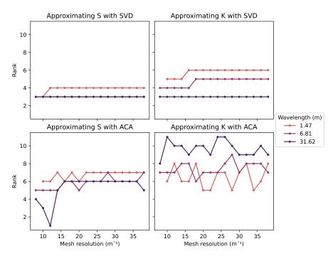
Figure 7: Rank of the best low-rank compression for a given error threshold, as a function of the mesh resolution, for two methods of low-rank compression (SVD and ACA) and two BEM matrices (S and K), for several wavelengths. Points for which the mesh resolution is insufficient for a given wavelength have been removed from the graph.
