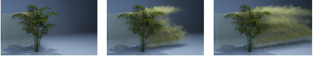
Fig. 5. Wind through a fern: A static 3D model of a fern is placed in a strong flow field, generating a complex wake (visualized with particles).
