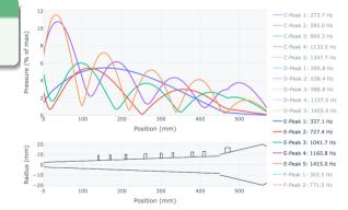
ContextPhysicsOpenwindTeachingConclusionActivity 2 : Tuning a specific resonance (for side holes instruments)
