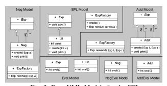
Fig. 3: Base UML Models for the EPL
