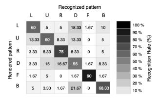
Fig. 5: Custom vibrotactile handle: perceptual experiment. Confusion matrix showing the recognition rates when activating each of the six motors (see also Fig. 1).
