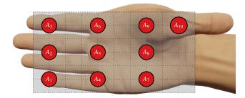
Figure 4: Actuators' matrix projected on a hand with approximative positions (positions may vary with hand morphology).
