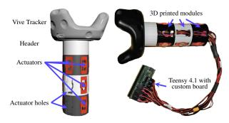
Figure 3: Views of the prototype. On the left, the frame of the controller, made of 3 modules, the header, and the *Vive Tracker*, fitted with the 10 actuators. In the center right, the actual prototype and the electronic board.
