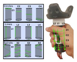
Figure 5: Matrix of the vibration patterns. On top, the circle patterns (C1 to C4), in the middle, the line patterns (L1 to L4), and at the bottom, the spiral patterns (S1 to S4).
