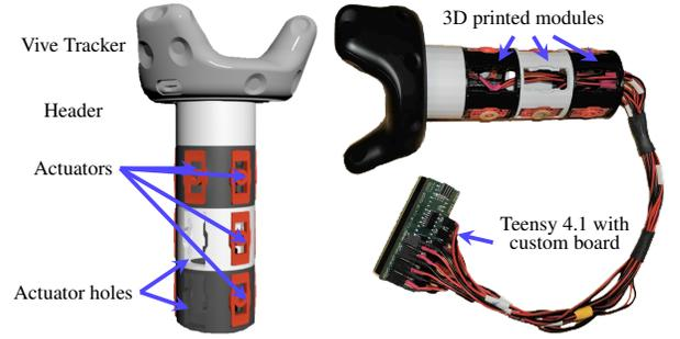
Figure 3: Views of the prototype. On the left, the frame of the controller, made of 3 modules, the header, and the *Vive Tracker*. In the center right, the actual prototype with 3D printed modules, actuators, and the electronic board.
