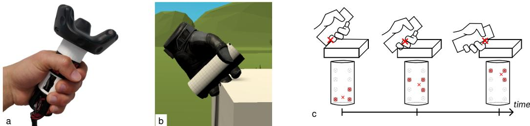
Figure 1: (a) *MultiVibes* prototype comprising 10 actuators in contact with the skin that can be controlled individually in amplitude and frequency. (b) Interaction with the edge of a virtual cube. (c) As the user slides the controller along the edge of the cube, they feel a phantom vibration point moving inside their hand according to the point of contact. The vibration point location is determined by the three closest actuators, controlled using our funneling model.
