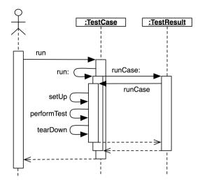
Figure 7-1 Running one test.
