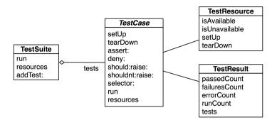
Figure 5-3 The four classes representing the core of SUnit.
