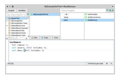
Figure 3-3 Running SUnit tests from the System Browser.
