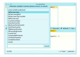
**Figure 4-2** Pharo class browser request actions to handle the fact that the class Counter is undefined.
