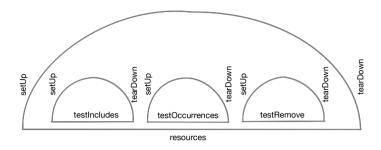
Figure 6-2 setUp and teardDown in action.
