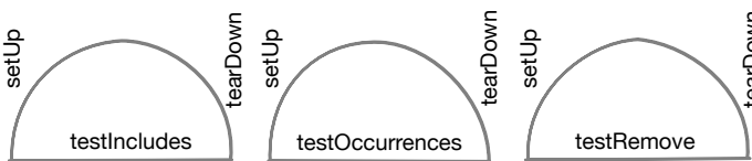
Figure 5-2 setUp and tearDown in action.
