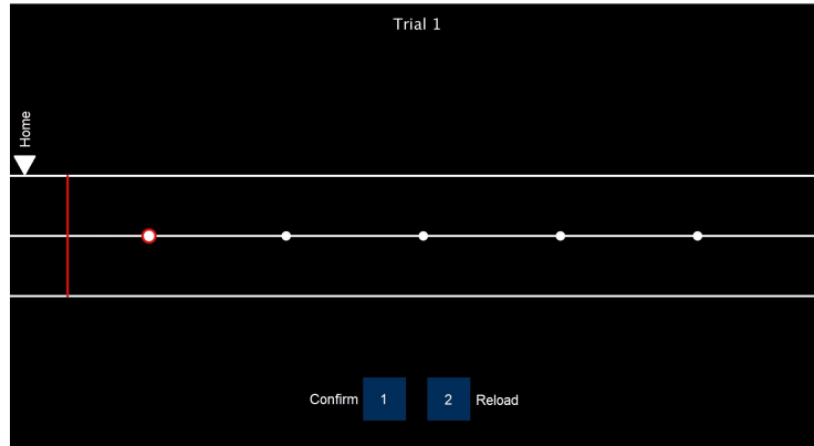
Fig. 3: The GUI used in the experiment. A vertical red cursor is controlled by the haptic knob; it moves along a virtual horizontal slider which hosts five round markers. At each trial, one marker is highlighted with the red color, thus becoming the current target. The blue squares are activated by pressing the corresponding buttons on the computer keyboard.
