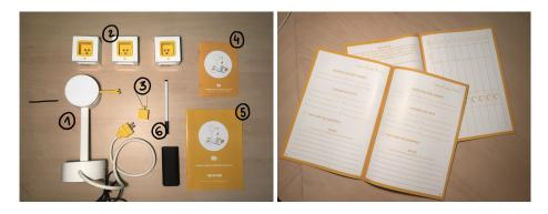
**Fig. 4.** The evaluation kit and diary: (1) RU, (2) three sockets, (3) weight, (4) instructions of use, (5) diary, (6) whiteboard marker and power bank
