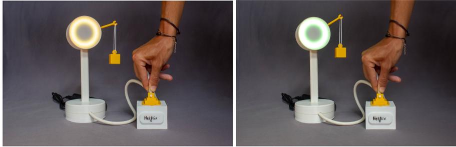
**Fig. 2.** The interaction for charging RU to the socket with the activity “Netfix” assigned to it. Yellow light (left) indicates that is charging. Green light (right) means fully charged
