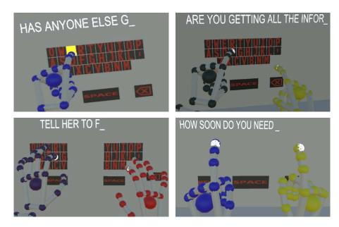
Fig. 1. Entering text using the normal keyboard with one hand (top left), the normal keyboard with two hands (top right), the split keyboard with two hands (bottom left), and the invisible keyboard (bottom right).
