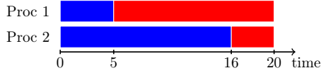
Fig. 1 Toy example with two processors, two successfully completed tasks (in blue) and two not-yet-completed tasks (in red) at time 20.
