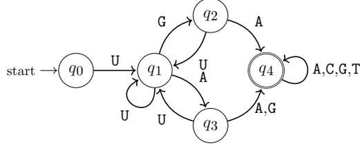
**Fig. 8** Sketch of the 5-state Deterministic finite “Aho-Corasick” automaton accepting the three stop codons UGA, UUA, UUG. We do not draw back-transitions to  $q_0$ , which occur implicitly for all not explicitly shown cases (i.e. A,C,G in  $q_0$ ; C in  $q_1$ , C,G in  $q_2$ ; and C in  $q_3$ ). To *forbid*, instead of accept, all of the three stop codons, we complement the language by making all states but  $q_4$  accepting.
