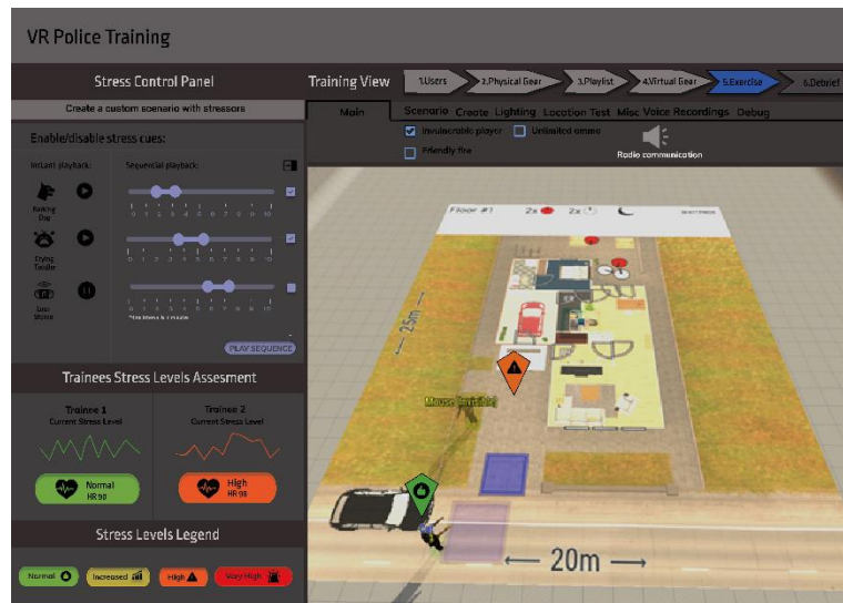
Fig. 1. Stress cue live editor showing stress levels of trainees and selected stress cues and control panel to add (1) single stress cues, (2) stress cues in parallel, or (3) in a sequence. Screens based on existing software by the VR partner RE-liON in SHOTPROS.
