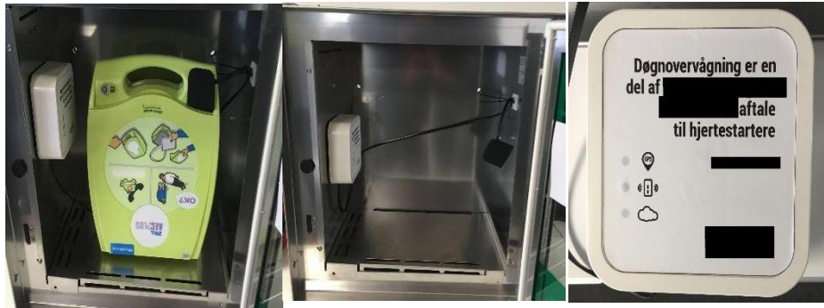
Fig. 4. Left: AED inside the cabinet. Middle: The monitoring unit and “optical eye.” Right: The monitoring unit.
