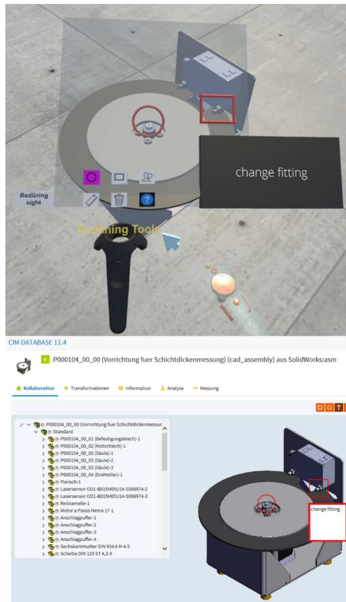
Fig. 3. VR redlining during creation and depiction in the PDM system CIM Database
