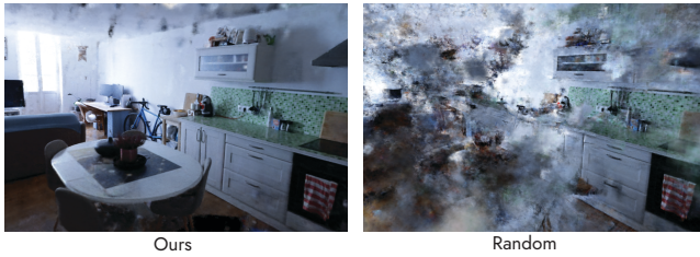
Figure 7: We also do a preliminary simulated evaluation of our method with a real scene, in which we captured approximately 1300 images, from which we exclude every 14th image and create a test-set. We use our algorithm to select the best 200 and we compared it against choosing 200 images at random. On average Our selection scored 16.4 PSNR while the random selection scored 13.8 PSNR.
