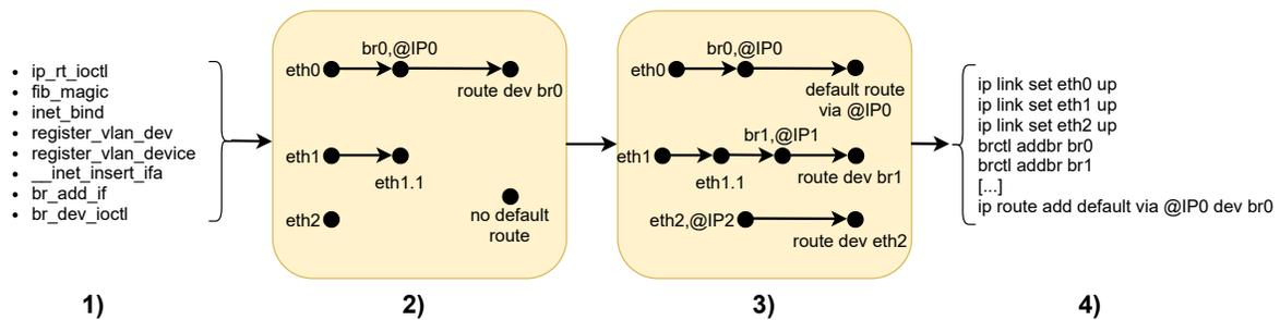
Fig. 4: Network configuration Enhancer (NCE) algorithm
