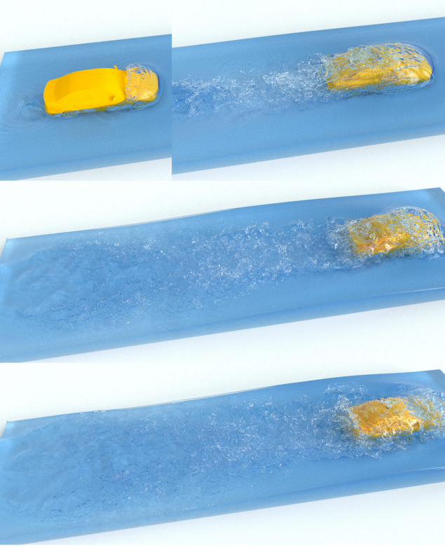
Fig. 7. Car in a flood. We simulate a car driving around 40mph through high water before coming to a stop; the usual “air bubble” forms in front of the car, and complex water patterns appear in the wake flow region.
