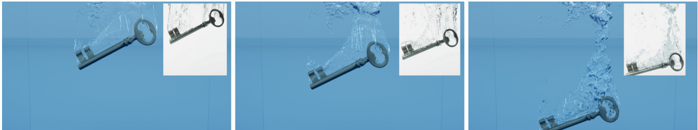
Fig. 1. Key Drop. In this paper, we propose a stable and efficient kinetic two-phase flow simulator which can handle complex fluid-solid coupling, like a skeleton key being dropped in water. The dynamics of the bubbles entrapped by the fall is well captured as the insets of a real experiment demonstrate.
