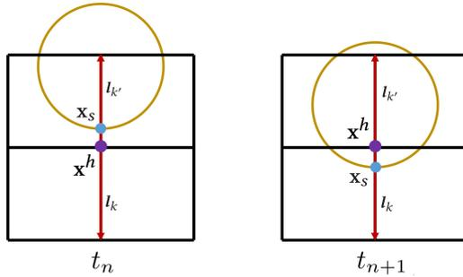
Fig. 13. **Dead cut-cells.** When phase grid node  $x^h$  gets covered by a solid (like the yellow disk here) between two time steps, it becomes a dead node, and its distributions  $h_k$  are then set to zero.
