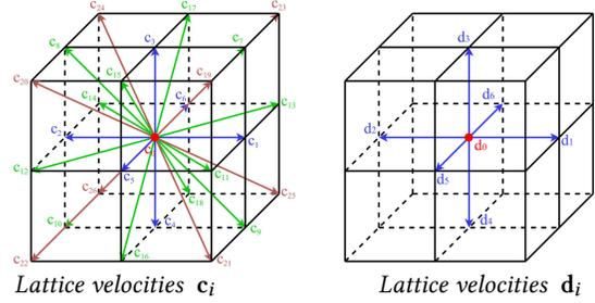
Fig. 3. **Lattice structures.** Flow velocities are stored and updated in time on a D3Q27 lattice (left) for high-accuracy with lattice weights  $w_i^c$ , while a simpler (and more memory-efficient) D3Q7 lattice structure (right) with lattice weights  $w_i^d$  suffices to encode the phase field.
