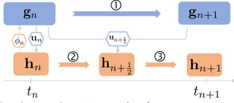
Fig. 10. **Time integration.** A time update from  $t_n$  to  $t_{n+1}$  is performed in three steps: (1) first, the flow equation is integrated using the phase field at time  $t_n$  (top); then the phase field is updated in two (2)+(3) substeps (bottom), first using the macroscopic velocity at time  $t_n$ , then using the average of the velocity at  $t_n$  and the one at  $t_{n+1}$ . Coupling between flow and phase field equations is indicated through hexagonal labels here.
