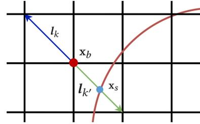
Fig. 6. **Hybrid moving bounce-back.** In the streaming step, we accommodate fluid-structure coupling through bounce-back: the distribution function at a node  $\mathbf{x}_b$  whose link  $l_k$  hits a solid boundary at an intersection point  $\mathbf{x}_s$  is made to bounce-back towards the opposite direction  $k$ , along with a momentum exchange due to the solid's speed.
