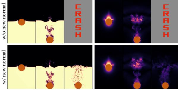
Fig. 12. **Ablation test for interface normal computation.** On this example of a ball dropping in a water tank (left: visualizing the phase field; right: visualizing the velocity field), if the normalized phase gradient is not handled through Eq. (17), the simulation crashes when the ball hits the bottom (top); with our new interface normal evaluation (and no other change in the simulation), the dynamics is properly captured (bottom).
