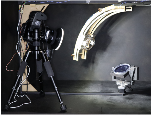
Capture tool to collect images of Flavobacteria [20]
