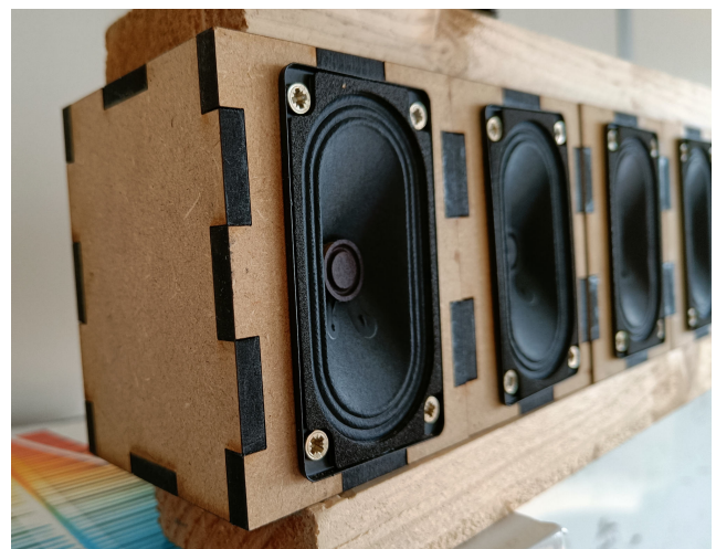
Figure 5: DIY speaker developed for our prototype WFS system.
