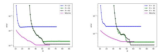
Figure 8: Frictionless Hertz test case, mixed method: RBM approximation errors. Right: displacement errors  $e_{N,R,\max}^{u}$  and  $e_{N,\max}^{u}$ ; Left: normal stress errors  $e_{N,R,\max}^{\lambda}$  and  $e_{N,\max}^{nn}$ .
