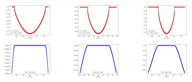
Figure 3: Frictionless Hertz test case, Nitsche's method (HF). Row 1:  $\sigma_{nn}(\boldsymbol{u}(\mu))$  and  $[P^n_{\gamma,g}(\mu;\boldsymbol{u}(\mu))]_-$ . Row 2:  $u_n(\mu) - g(\mu)$ . Column 1:  $\mu = 0.7$ m. Column 2:  $\mu = 1.0$ m. Column 3:  $\mu = 1.3$ m.
