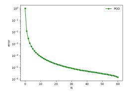
Figure 10: Frictional Hertz test case, Nitsche's method: Relative POD projection error  $e_{POD}(N)$ as function of N, for  $|\mathcal{D}_{train}| = 61$ .
