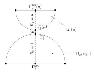
Figure 1: Frictionless Hertz test case: Configuration.
