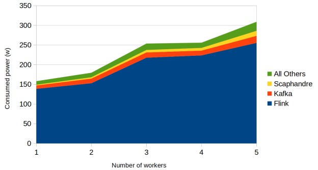
Fig. 10. Impact of consolidation strategies when processing a workload of 50,000 records/second.
