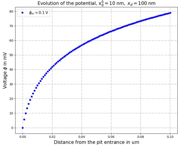
Figure 4.19: Potential profile in 100 nm deep pit.
