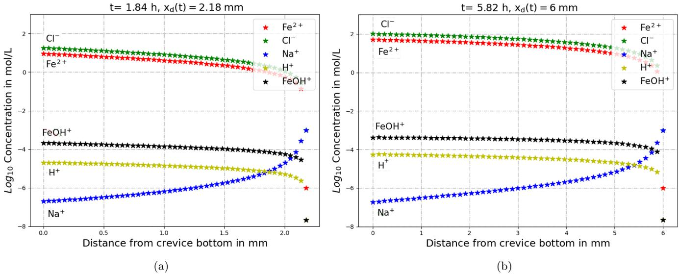
Figure 4.2: Evolution of the solution chemistry in the crevice given by the developed model with moving interface for the initial data :  $\phi_m = 0.04 \text{ V}|_{\text{NHE}}$ ,  $C_{\text{Fe}^{2+}}^0 = 10^{-6} \text{ mol/L}$ ,  $C_{\text{NaCl}}^0 = 10^{-3} \text{ mol/L}$  and  $x_d(0) = 2 \text{ mm}$ .
