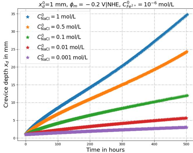
Figure 4.4: Influence of the initial concentration of chloride ions on the time evolution of the crevice depth.
