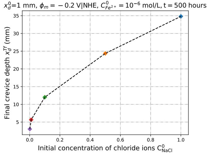
Figure 4.5: Evolution of the crevice depth after 500 hours of the crevice propagation for different values of initial chloride concentrations  $C_{\text{NaCl}}^0$  (with  $x_d^0 = 1 \text{ mm}$ ,  $\phi_m = -0.2 \text{ V|NHE}$ ,  $C_{\text{Fe}^{2+}}^0 = 10^{-6} \text{ mol/L}$ ,  $t = 500 \text{ hours}$ ).
