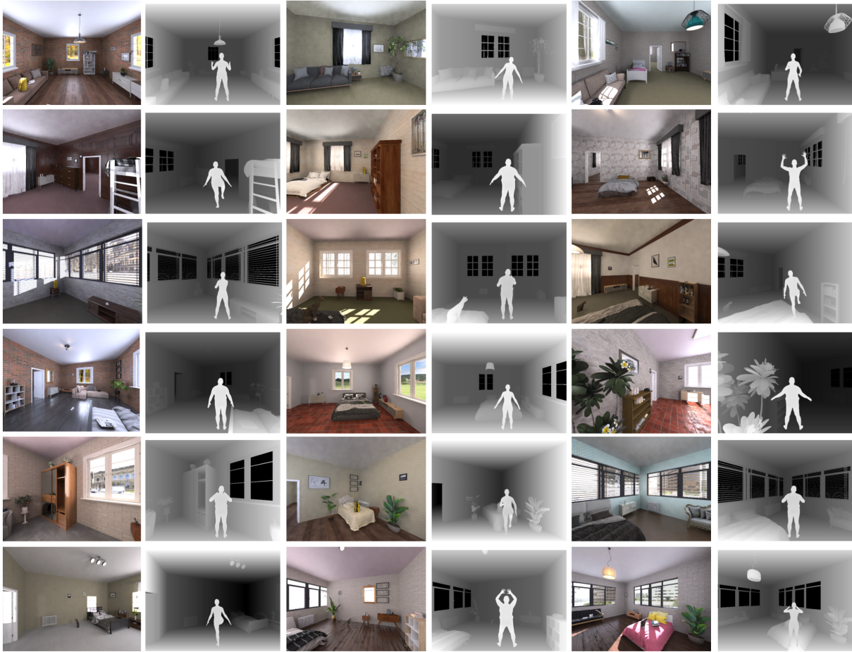
Fig. 3. Examples of our synthetic dataset. For each scene, the left image stands for the background image and the right one depicts an example of the final depth input after adding the character depth image.
