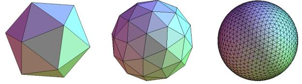
**Figure 3: The first one is the original icosahedron (20 faces). The second and the third ones are the geodesic structures with tessellation frequencies  $n = 2$  and  $n = 10$  respectively.**
