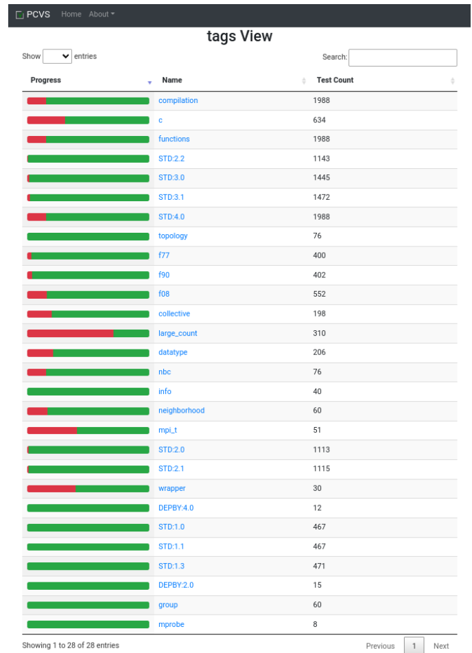
Figure 7: Sample output from the PCVS web-based result explorer, showing the tag-based view of MPC’s result.
