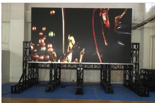
Fig. 1. 200-inch LED display used for the experiment.
