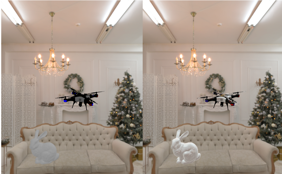
Fig. 5. Left: rendering of XR scene with inconsistent lighting. Right: relighting of XR scene with consistent environment lighting.
