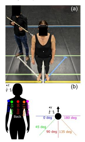
Figure 1: (a) Illustrative picture taken as the participant was about to receive a perturbation with an angle of 45 deg. (b) Angles of application location of the perturbations.
