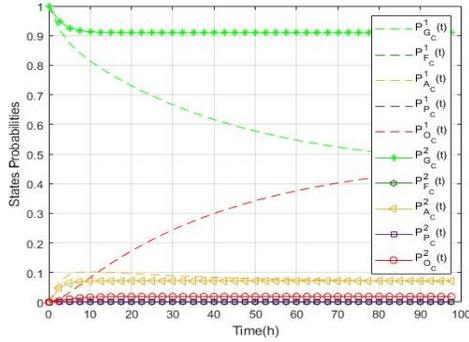
Fig. 6: Evolution of radio coverage states probabilities (S1, S2):  $P_{i_C}^1$  and  $P_{i_C}^2$  stand for probability of state  $i \in S$  of coverage indicator in S1 and in S2 scenarios, respectively.
