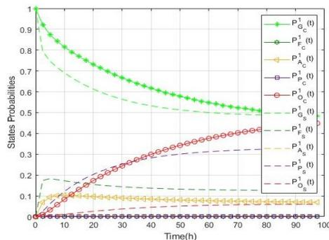
Fig. 7: Evolution of coverage vs. service states probabilities (S1):  $P_{i_C}^1$  and  $P_{i_S}^1$  stand for probability of state  $i \in S$  of coverage and service indicators, respectively in S1 scenario.
