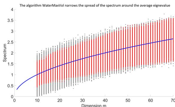
Fig. 4. From a  $d \times n$  Gaussian matrix  $A$ , spectrum of  $d \times m$  extracted random matrices  $C$  (grey) and spectrum of  $d \times m$  extracted submatrices  $B$  obtained by the proposed WaterMaxVol (red), as a function of the number of columns  $m$ . Mean curve  $\sqrt{m/d}$  is in blue.  $d = 10$ ,  $n = 100$ , 100 independent samples superimposed.
