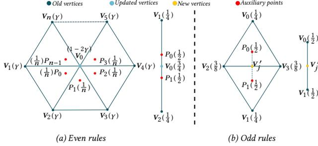
Fig. 13. Subdivision rules for even and odd interior and boundary vertices. First, sample  $\omega$  and  $z$  (using Equation (19)) at the red points  $P_i$ , using the barycentric weights specified in parentheses next to the vertices. Finally, extrapolate  $z(P_i)$  to the upsampled vertex (blue or yellow) using an analogous approach to Equation (21), and average these extrapolations using the weights in parentheses next to the  $P_i$ .
