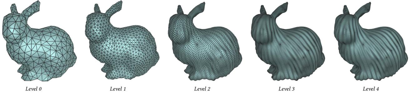
Fig. 14. We successively Loop-upsample the Stanford bunny, alongside the  $\mathbf{z}$  and  $\omega$  of a CWF on the bunny, and render the resulting displaced surface. After several rounds of subdivision, the wrinkle pattern appears and is stable under additional iterations of subdivision.
