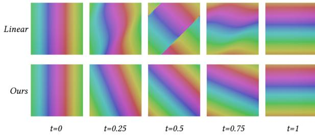
Fig. 8. Failure of linear interpolation given boundary conditions  $z_0 = \exp ix$  and  $z_1 = \exp iy$ . We show the phase patterns at several intermediate frames using linear interpolation (top row) and our proposed interpolant (bottom row). Notice that linear interpolation introduces severe artifacts in the wrinkle pattern: wrinkles shear and degenerate along a sharp line midway through the interpolation.
