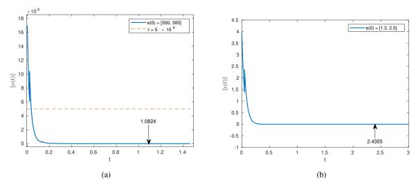
Figure 2: (a) Nearly Fixed-time convergence of system (49) to a  $\delta$ -nbh of the origin.(b) FTS of system (49) with ADT condition.
