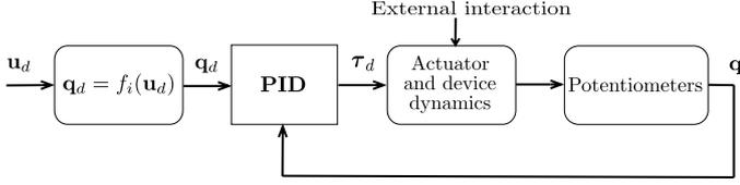
Figure 11: Position control system. The reference configuration is provided in the end-effector configuration space  $\mathbf{u}_d$ . The inverse kinematics procedure described in Sec. 3 allows to convert the desired configuration in the joint space. Finally, a PID controller is implemented, providing the desired motor torque  $\tau_d$ . The actual joint configuration is measured by the potentiometers placed on the device active joints (C, D, E, F – see Fig. 2).
